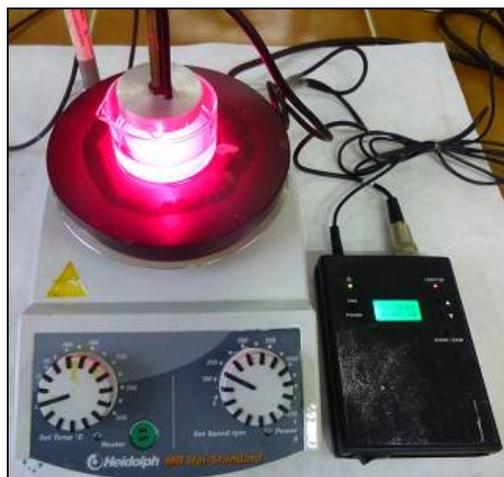
Figure 1: Testing of photocatalytic effect of fabrics
